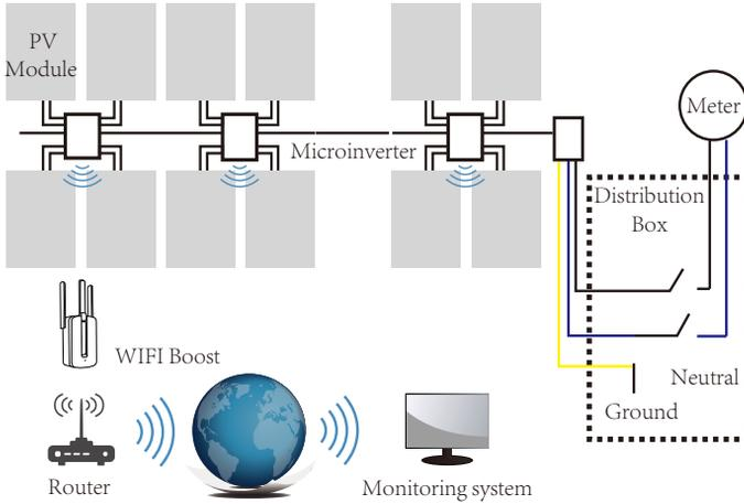
**NOTE:** If the wireless signal in the area where the microinverter is weak is weak, it is necessary to add a wifi signal booster at a suitable place between the router and the microinverter.
