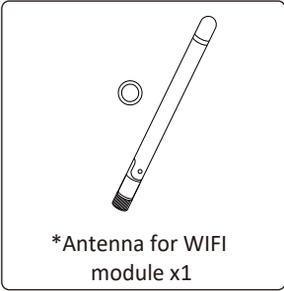
\* This antenna is for microinverter that has built-in wifi module.
